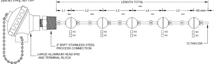
The above sensors have been subject to the following test compliance with AS/NZS 60079.11:2006 Explosive Atmospheres Part 11 Equipment Protection by intrinsic safety 'i '. Section 6.3.12 Dielectric strength requirement "500 VAC RMS TEST VOLTAGE OF INSULATION RESISTANCE BETWEEN CONDUCTORS OR CONDUCTORS & SHEATH FOR 2 MINUTES"
