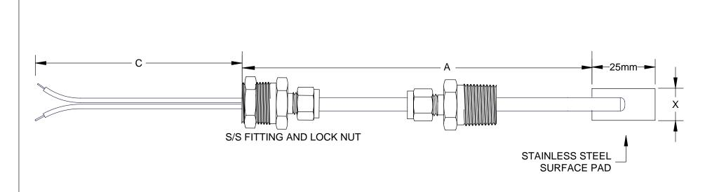
OPTION - Ex ia Compliance with ANSI AS/NZS 60079. 11.2006 Explosive Atmospheres, Intrinsic safety Ex ia (1047 RTD & TC) TYPE K THERMOCOUPLE TYPE J THERMOCOUPLE TYPE T THERMOCOUPLE MIMS TYPE N THERMOCOUPLE AND DUAL COMPRESSION FITTINGS 3 WIRE RTD PT100 TC05 STYLE 4 WIRE RTD PT100
