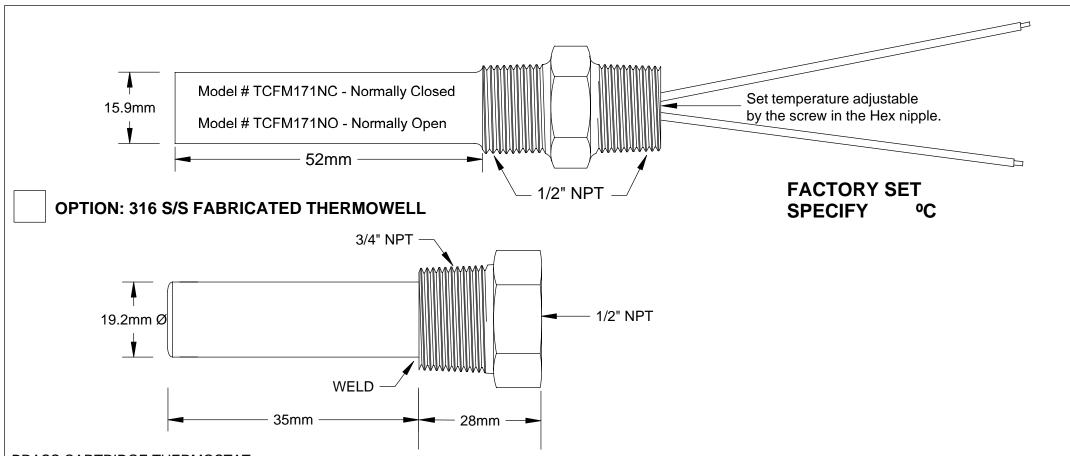
BRASS CARTRIDGE THERMOSTAT Adjustable thermostat Range: 0 to 250°C
