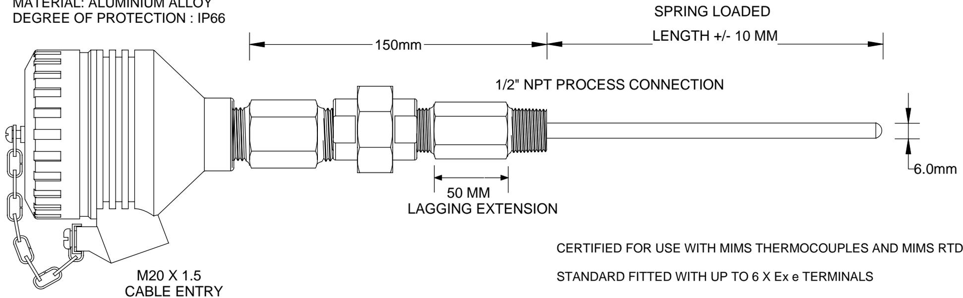
CERTIFIED FOR USE WITH MIMS THERMOCOUPLES AND MIMS RTD SENSORS
